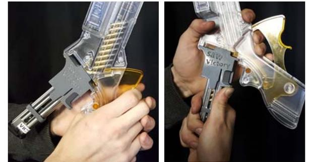
Be sure to have 10 shells lined up before loading and hold loader vertical.
