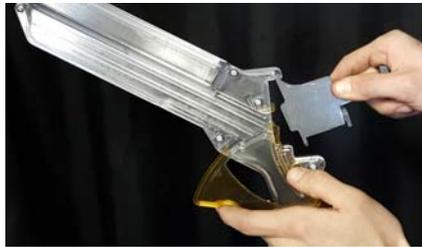
Insert your magazine through the small ring into the adapter until it latches into notch. The follower of your magazine will be pushed down when this is done
